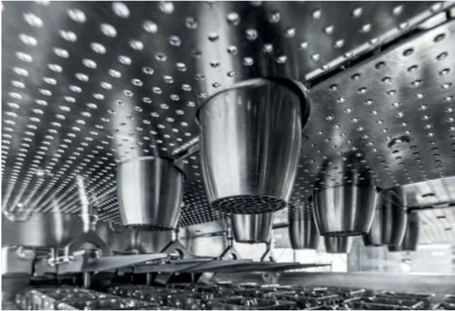
Fig. 5: The optional combi-filler of the E-PS120A allows many different products to be filled on the same machine – including high-viscosity liquids such as smoothies or drinks with fruit particles.
