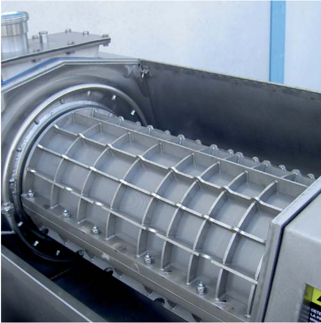
When prime juice is 'finished', pulp level is reduced in the juice.
