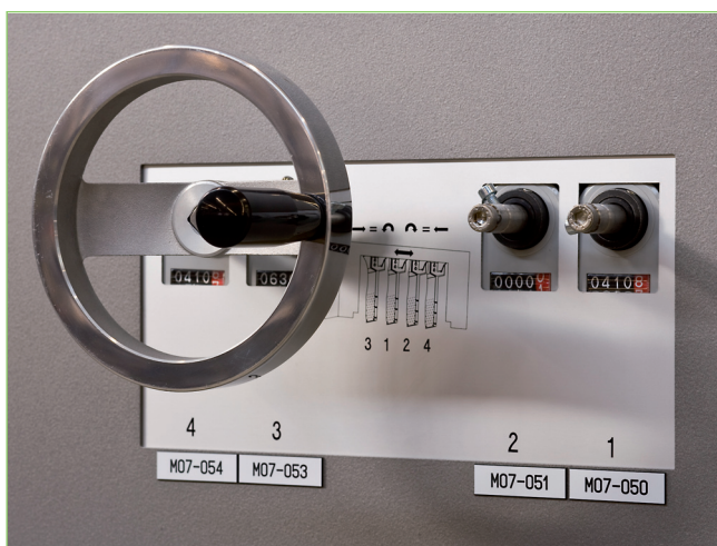
Easily adjustable in both height and width, hot air nozzles provide optimum shrink quality.
