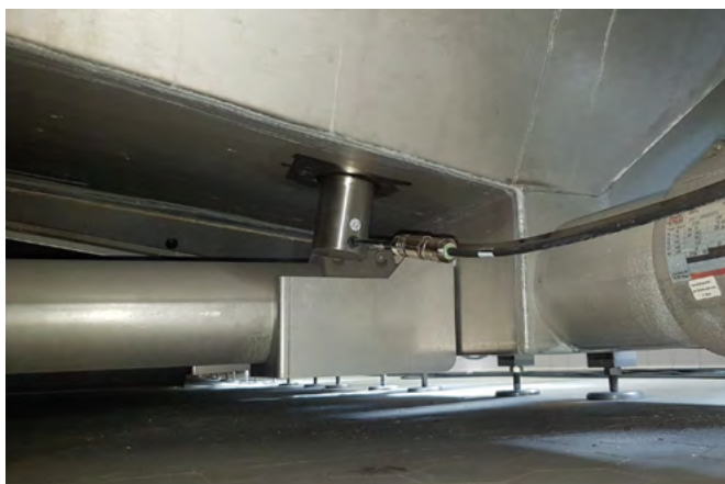
Installation of ultrasonic technology on a pasteurizer.
